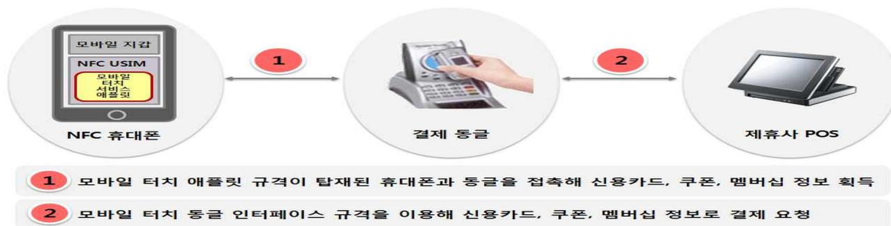
1. When the cell phone with the mobile touch applet standard touches the dongle, it acquires credit card, coupon and membership information.
